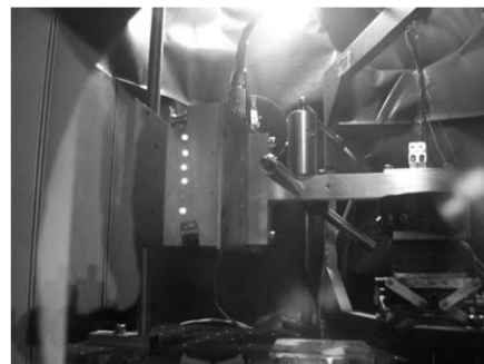
Fig. 25 The ms-LPT after assembly and during tests in vacuum. At right, the operating device is mounted on a torsion pendulum to measure thrust in vacuum (see [4]); used with permission of the American Institute of Physics, copyright 2007.
